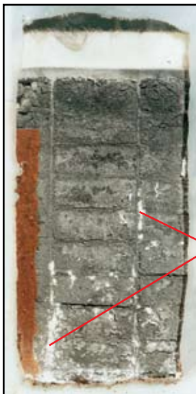
White crystallized lead sulfate can be easily seen on this battery plate. The plate was deeply discharged. Discharge time was just over 13 minutes
